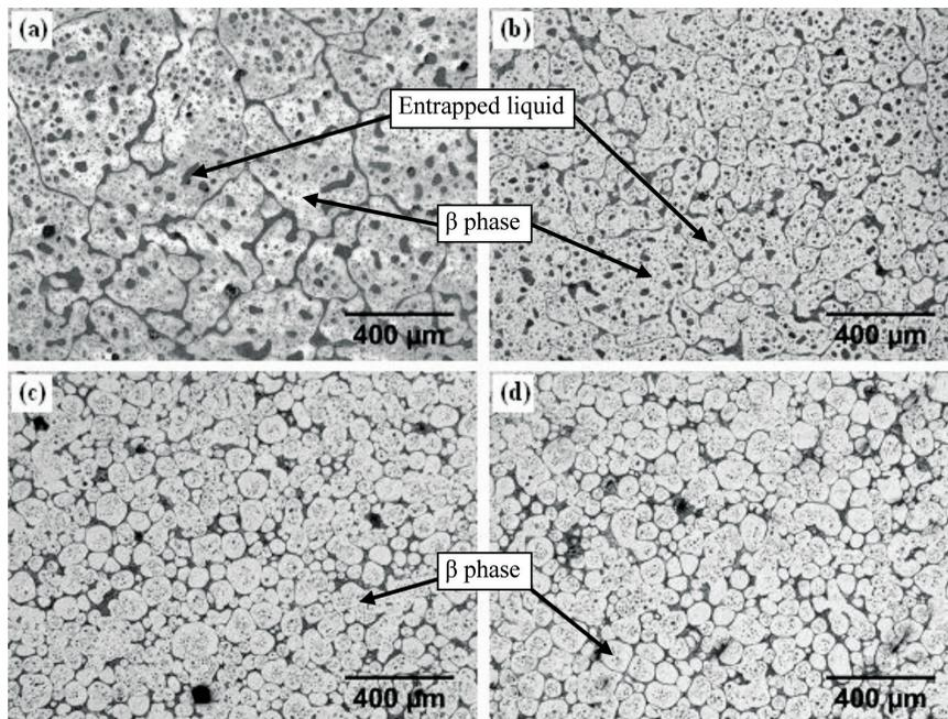
Fig. 4: Microstructure of Zn-22Al subjected to partial re-melting at 438°C for 1 hour on (a) as-cast sample, and on the samples which have previously solution treated at 315°C for (b) 1.5hrs, (c) 3 hrs, and (d) 5 hrs.
