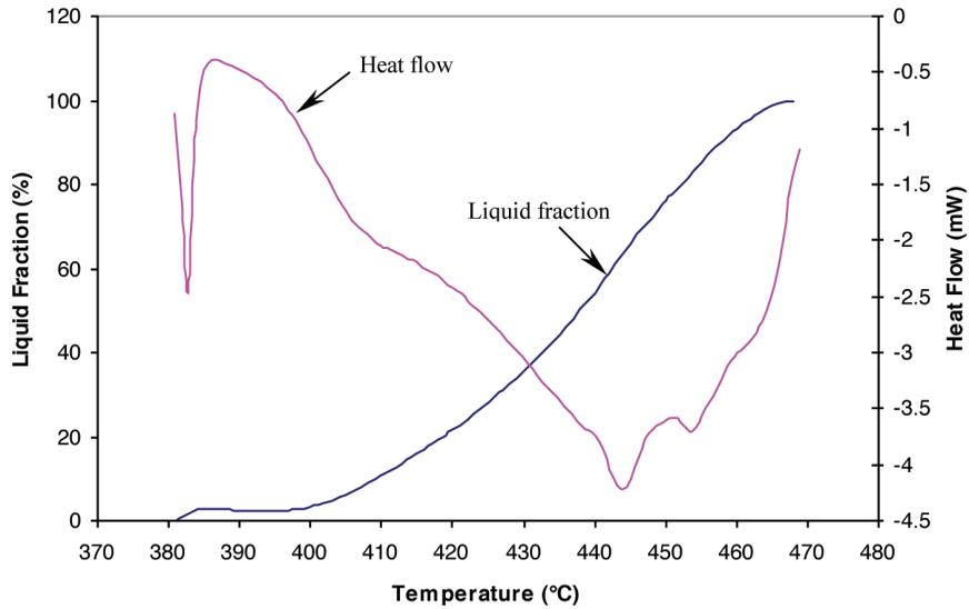
Fig. 3: DSC and liquid fraction curve of Zn-22Al
